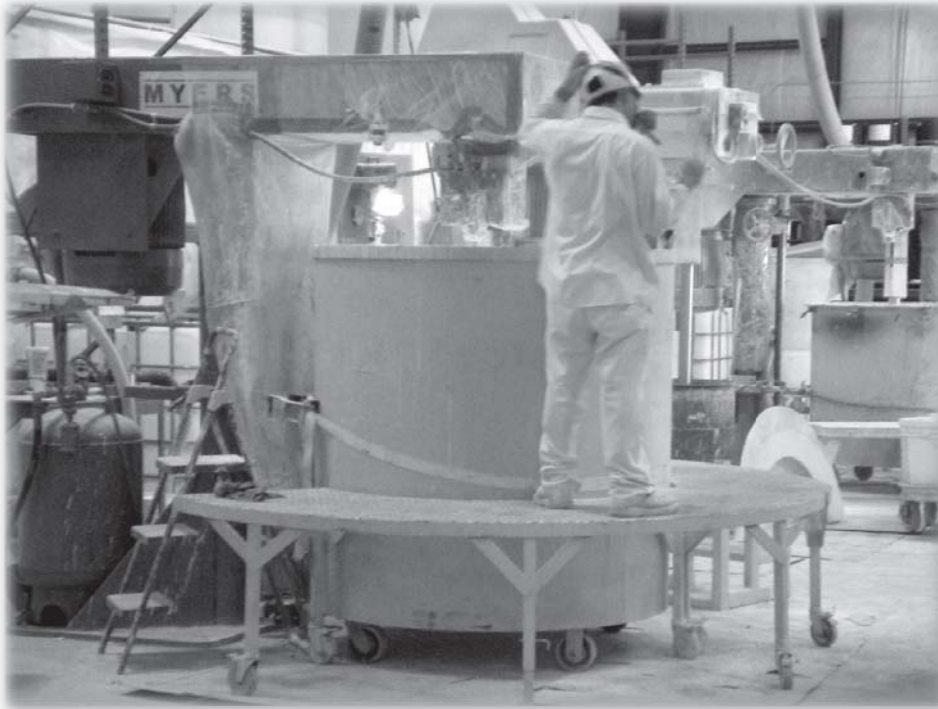
Danny Portillo begins a new batch in Elastek's newest 560-gallon super disperser.
