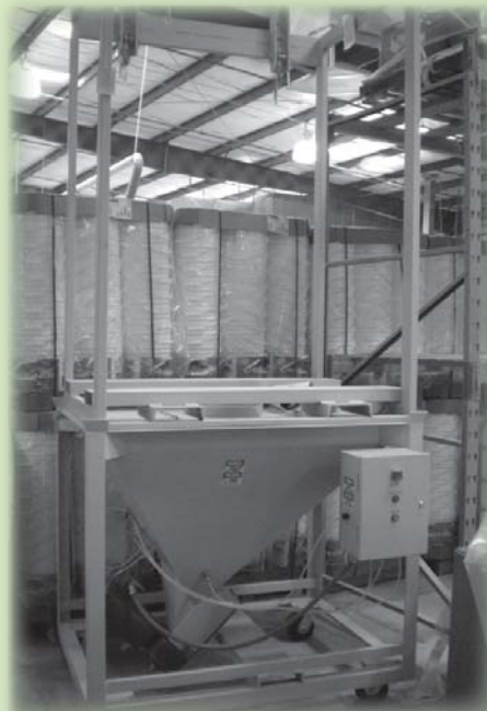
The new bulk powder feeder (above) will save on heavy lifting by placing the measured powders required into the disperser tanks.
