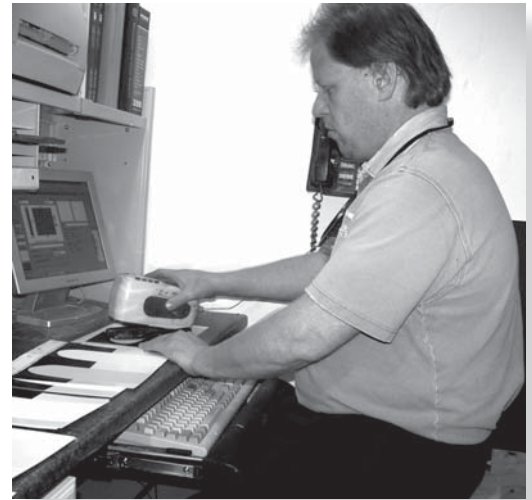
Jerry Rockwell measures the reflectivity of a coating that has been drawn-down onto a Leneta card. The instrument used is a spherical spectrophotometer.
